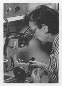
**MECHANICAL WINDER**, operated by Lois Donaghy (2133), has already placed 900 turns of No. 50 wire onto a core. Six wires are attached and numbered.
